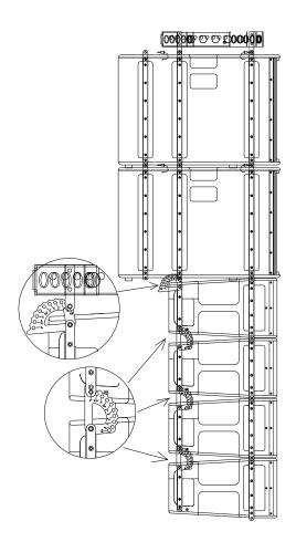
Fig.32. X-210 + X-215W flying, flat Line Array
