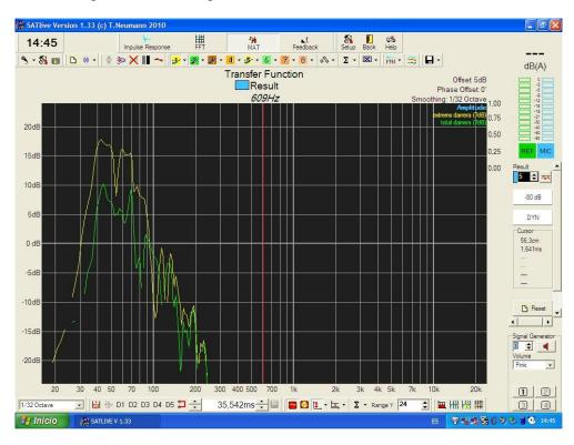
**Fig.22c. X218W** total back energy rejection. Yellow curve without central cardioid subwoofer; green curve adding central cardioid subwoofer.
