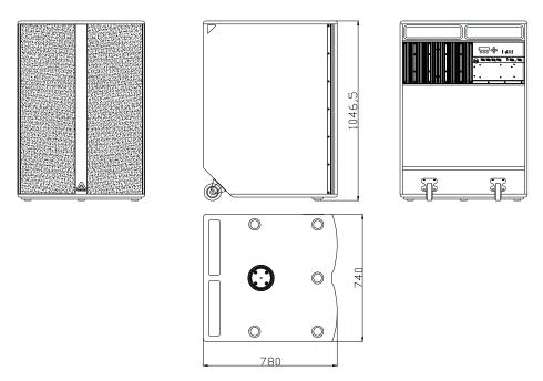
Fig.14. X-218W cabinet. External dimensions
