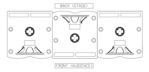
Fig.20. Cardioid configuration for X-218W subwoofer
