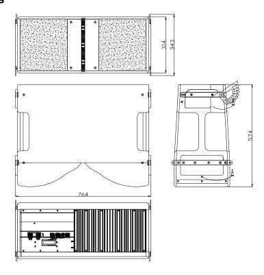
Fig.10. X-210 cabinet. External dimensions
