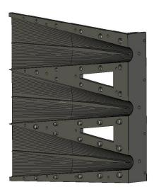
**Fig.3.** High frequency waveguide (half piece)
