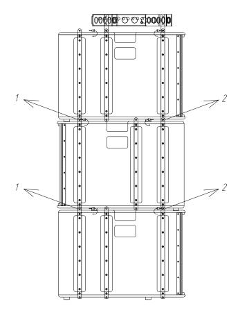
Fig.31. X-215W Flying, three units in cardioid configuration
