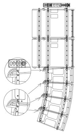
Fig.33. X-210 + X-215W Flying, curved Line Array
