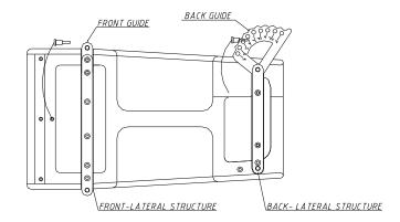
Fig.24. Flying hardware (lateral view)
