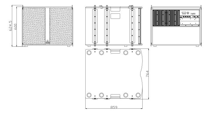
Fig.11. X-215W cabinet. External dimensions
