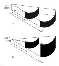
Fig.7.Cylindrical wave (A) vs Spherical wave (B)
