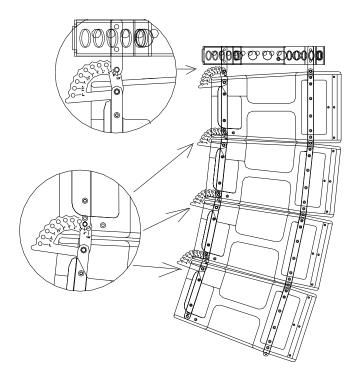
Fig.29. X-210 Flying. 6° Curved Line Array
