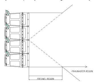
Fig.5. Limits of Fresnel-Fraunhofer Regions
