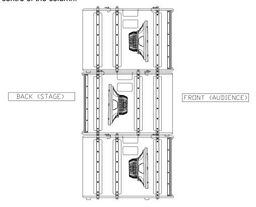
Fig.19. Cardioid configuration for X-215W subwoofer
