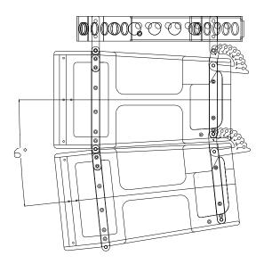
Fig.4. Tilt angle between cabinets (6° maximum)
