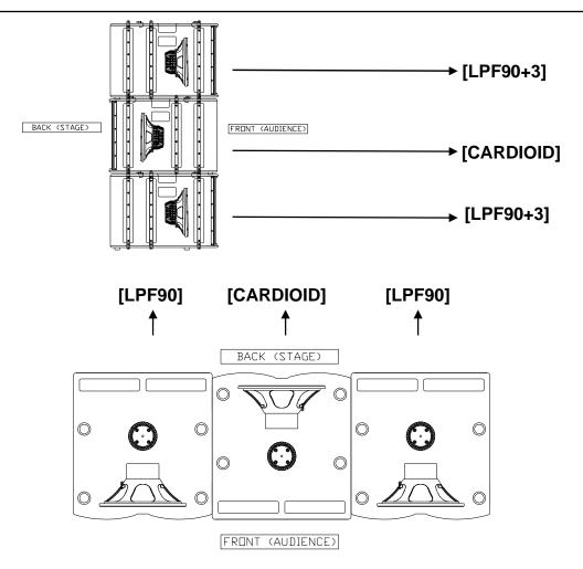
Fig.21. Presets for cardioid configuration
